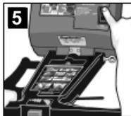
Fill the LOWER tank C with the cleaning solution you just mixed by pouring through the white filter screen. Machine is full when liquid halfway covers filter screen. (ILLUS.2)
