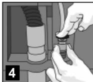
Lower the retaining wire A and remove the white UPPER tank B.
