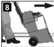
Plug in the power cord and position the machine. Refer to label on top of the machine E. Press the "ON" switch for CARPET cleaning on the top of the machine (ILLUS.5).
